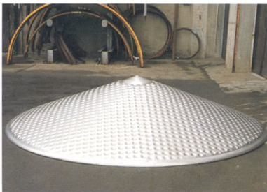
■ Detail of conical base with Thermoplate.
