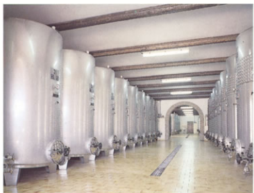
■ Group of normal, refrigerated tanks.
